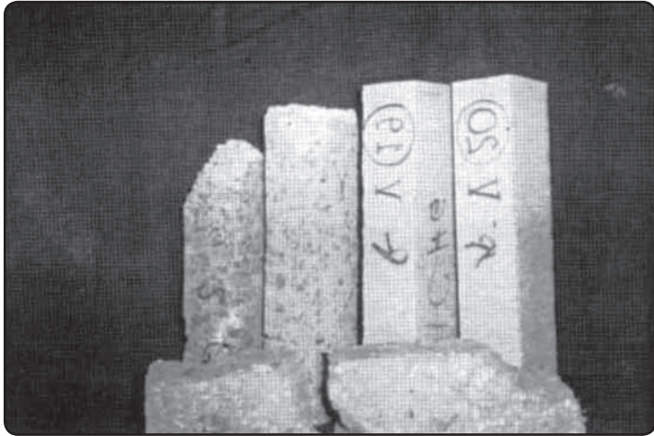
FIGURE 9: New granite and new precast concrete samples subjected to freeze/thaw testing.
