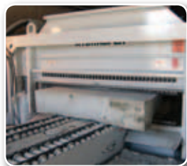
The slabs are cut to the required thickness. A hydraulic splitter is then used to cut these slabs into curbing.
